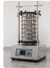
Sieve Shaker For particle size distribution analysis
