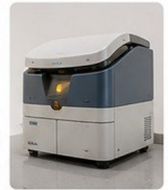
XRF Spectrometer For chemical composition analysis
