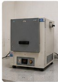
Muffle Furnace For loss on ignition test (LOI)
